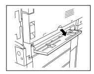
Adjust the paper guides to the size of the paper, and then load the paper so that the front side of the paper (the side facing up when the package was unwrapped) faces down. Lightly slide the paper into the feed slot as much as possible so that it is ready to be fed into the copier.
